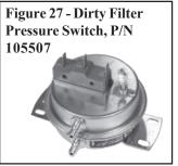
switch is only on systems with an optional console that includes a dirty filter light. The pressure switch is set during installation so that the light will be activated at approximately 50% filter blockage. Contacts should close at .17 to 5.0" w.c.  $\pm$  .05" w.c.
